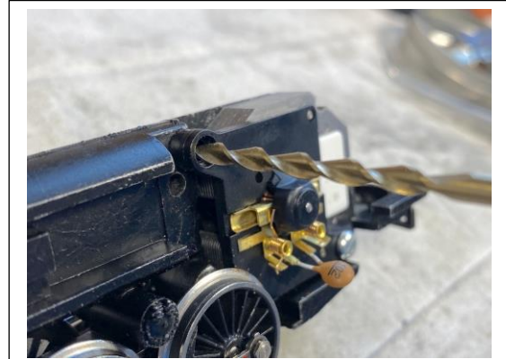
Fig. 3 - Finding where to drill
