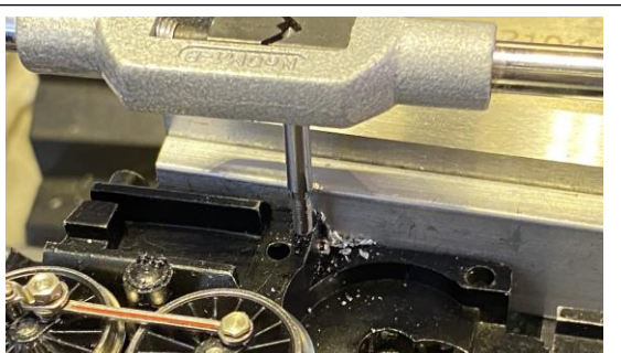
Fig. 6 - Tapping the threads
