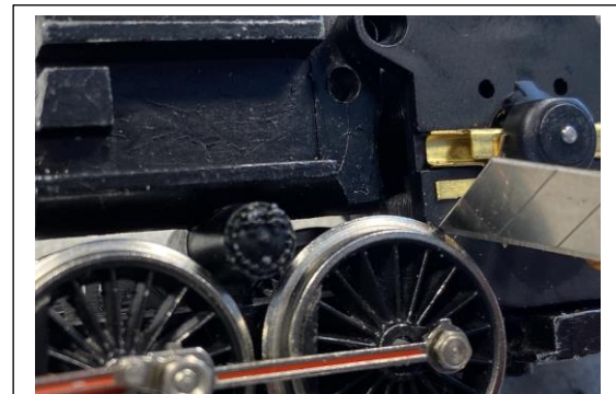
Fig. 5 - Scoring a line for clearance
